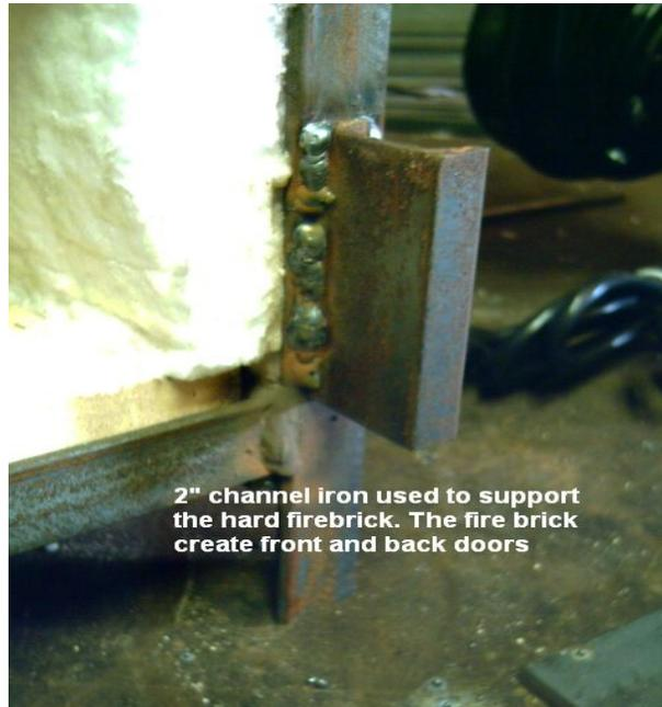
2" channel iron used to support the hard firebrick. The fire brick create front and back doors
