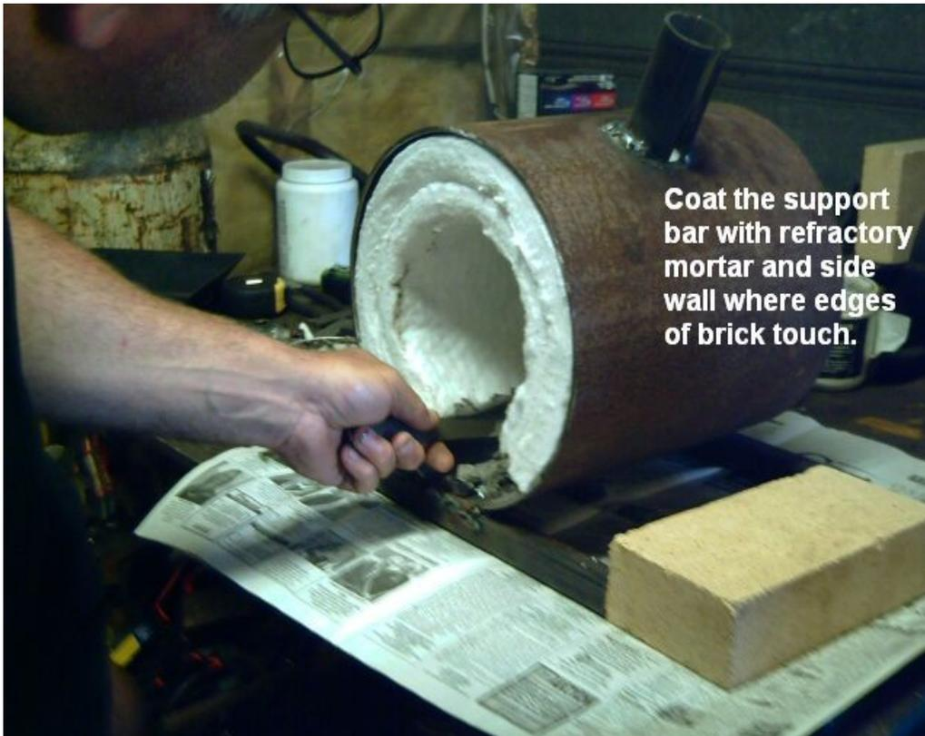
as to not disturb the Kaowool. Large brick first. Mortar the inner ends of the bricks and set the smaller one onto the waiting mortar. Please note you do not need to fill the gap between the support bar and the side wall. Just the edges of the brick and the top of the center bar.
