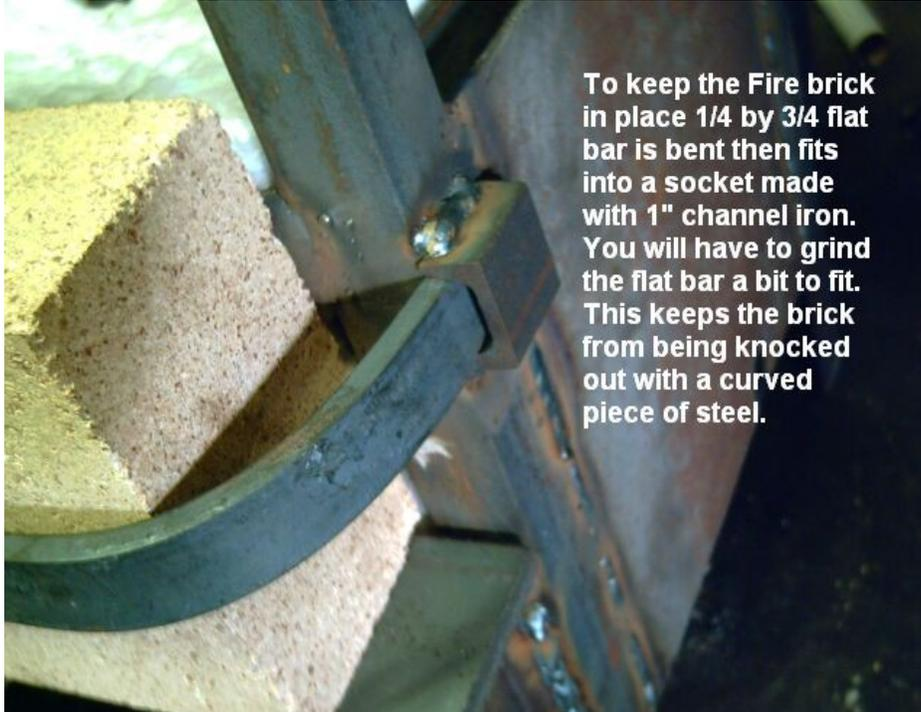
To keep the Fire brick in place 1/4 by 3/4 flat bar is bent then fits into a socket made with 1" channel iron. You will have to grind the flat bar a bit to fit. This keeps the brick from being knocked out with a curved piece of steel.
