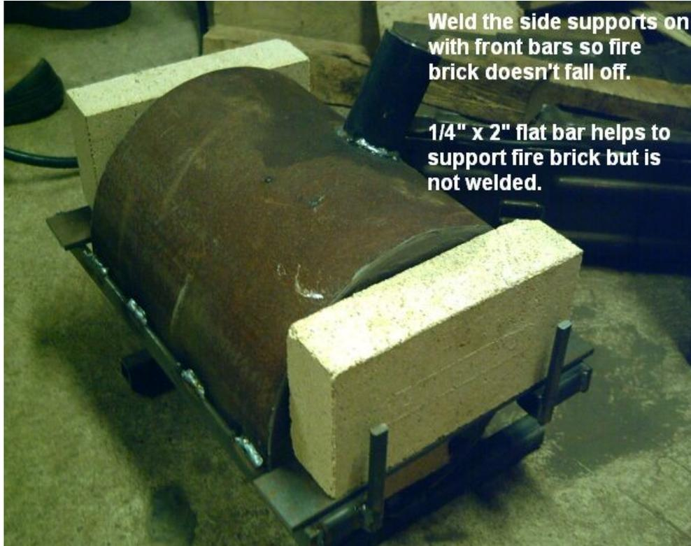
Weld the side supports on with front bars so fire brick doesn't fall off.
