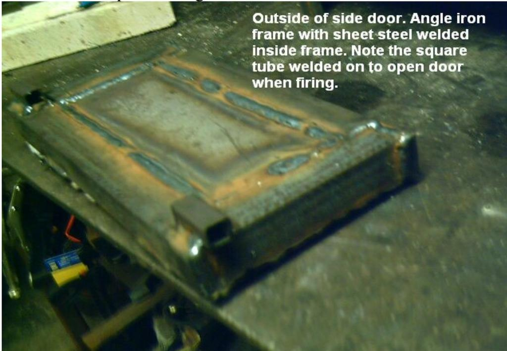
The idea behind this tube is that it gives you a place to put a square bar in while the forge is running to open the door if you have to put an odd shaped piece in for heating.
