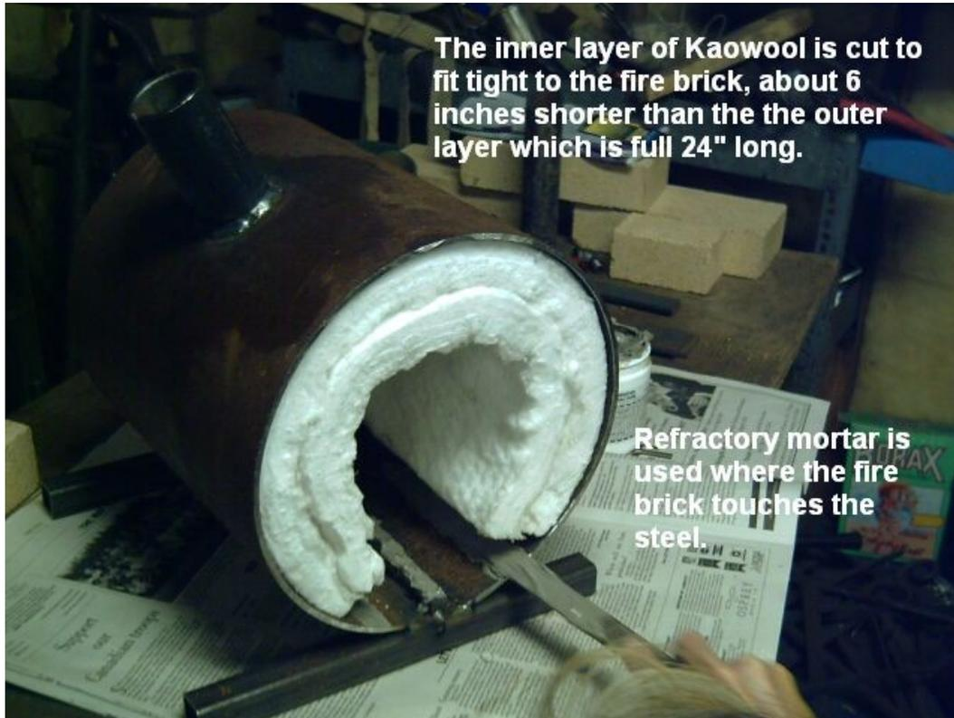
Once the fire bricks are set use a hacksaw blade to cut the Fibrofax from underneath the burner socket. I do this by gently forcing the blade through the insulation then slowly working the blade up and down cutting around the inside of the hole rubbing against the metal all the time. The hole you make should be slightly conic in shape with the large end of the cone being closest to the chamber. The 1 ¼ inch pipe should slide in with no trouble.
