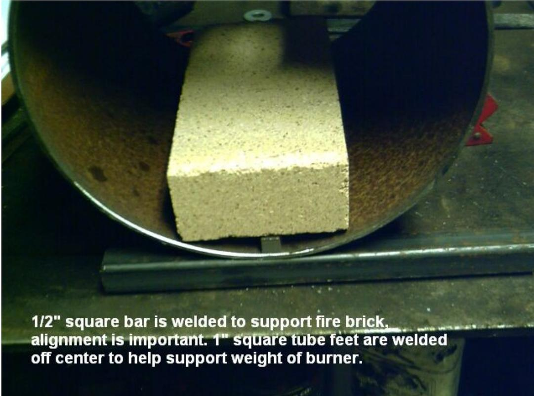
**1/2" square bar is welded to support fire brick, alignment is important. 1" square tube feet are welded off center to help support weight of burner.**
