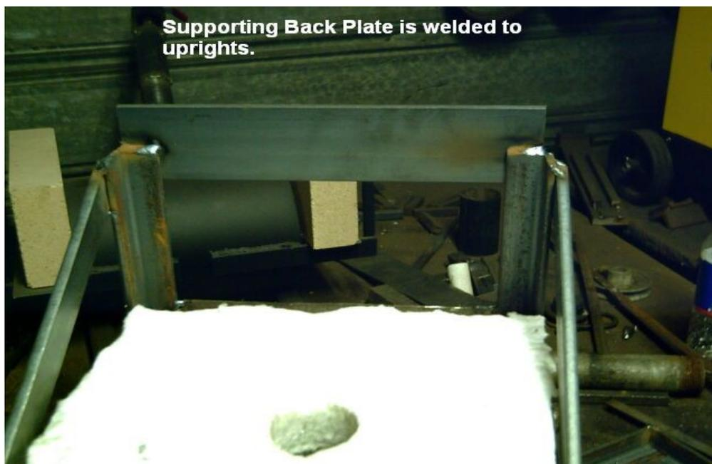
The supporting back plate is welded into position. In the photo I used ¼ x 2 as I cut my
