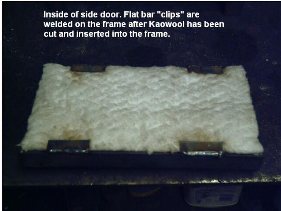
The frame of the door was previously constructed with the sheet steel welded in. Now cut a piece of Kaowool or Fibrofax that is slightly over size to fit in the door. Gently pack it in to the door as shown. Then weld on short  $1/8$  th x  $3/4$  x 2 inch flat bar strips to keep it in place. Make sure none of the weld over hangs the edges. Grind smooth if need be.
