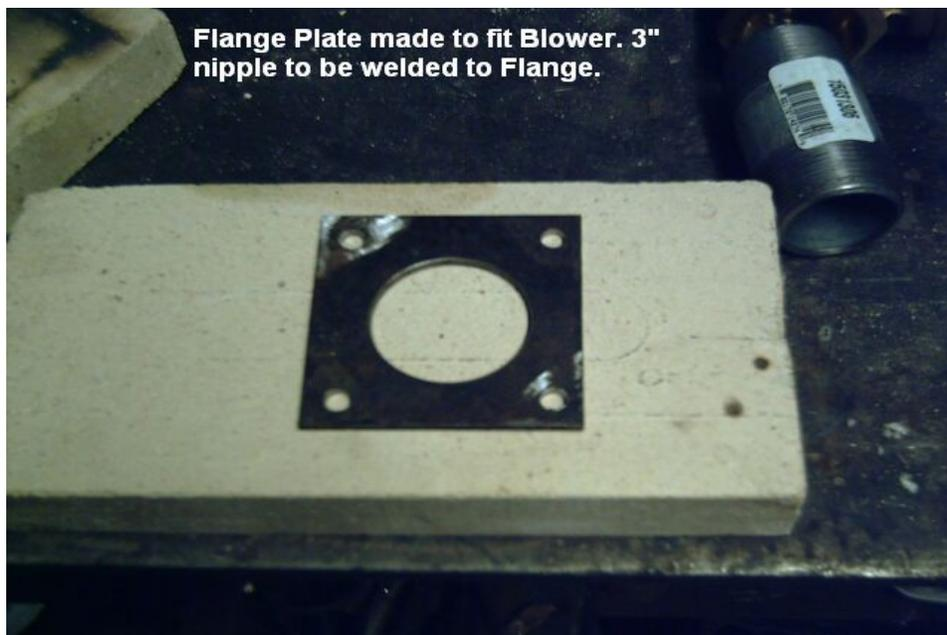
Flange Plate made to fit Blower. 3" nipple to be welded to Flange.
