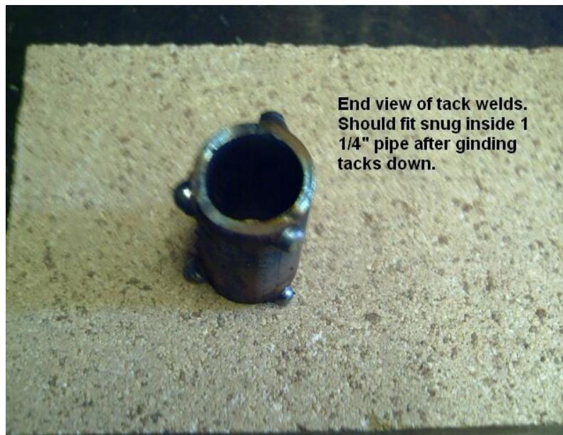
The smaller pipe is place inside the short end of the elbow pipe and tack welded on top of the tack weld to the wall.
