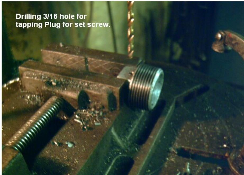
This is where you will thread using 1/4 inch tap for a set screw. This hole only needs to go through to the larger hole you drilled previously perpendicular to this one.
