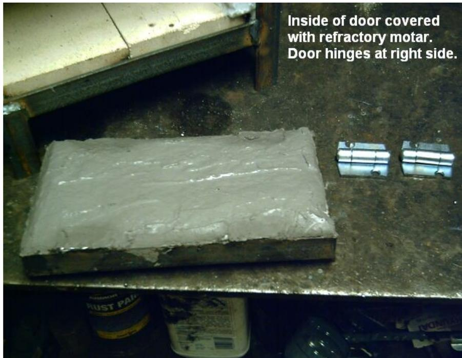
The above photo shows the inside of the door and the Kaowool coated with the refractory mortar. Follow the same procedure for drying and slow firing as in the pipe forge. You could also slow bake this in your oven or toaster oven at about 400 degrees for an hour to dry it out.
