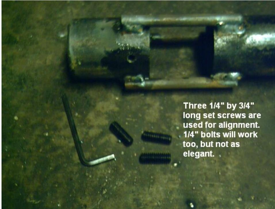
At this point the burner is complete except for the orifice.
