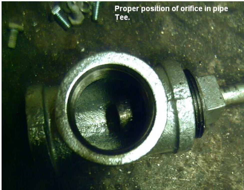
The nipple is then T-Taped or pipe compound and the cap threaded on. Then pass the free end through the whole drilled in the plug. Thread the plug into the Tee as shown above so that the end of the cap (seen inside the tee) is little more than half way back from the opposite side opening. Use the set screw to lock the orifice in place. The cap acts as an added safety feature if the set screw ever loosens up it will prevent the orifice from falling out of the Tee.
