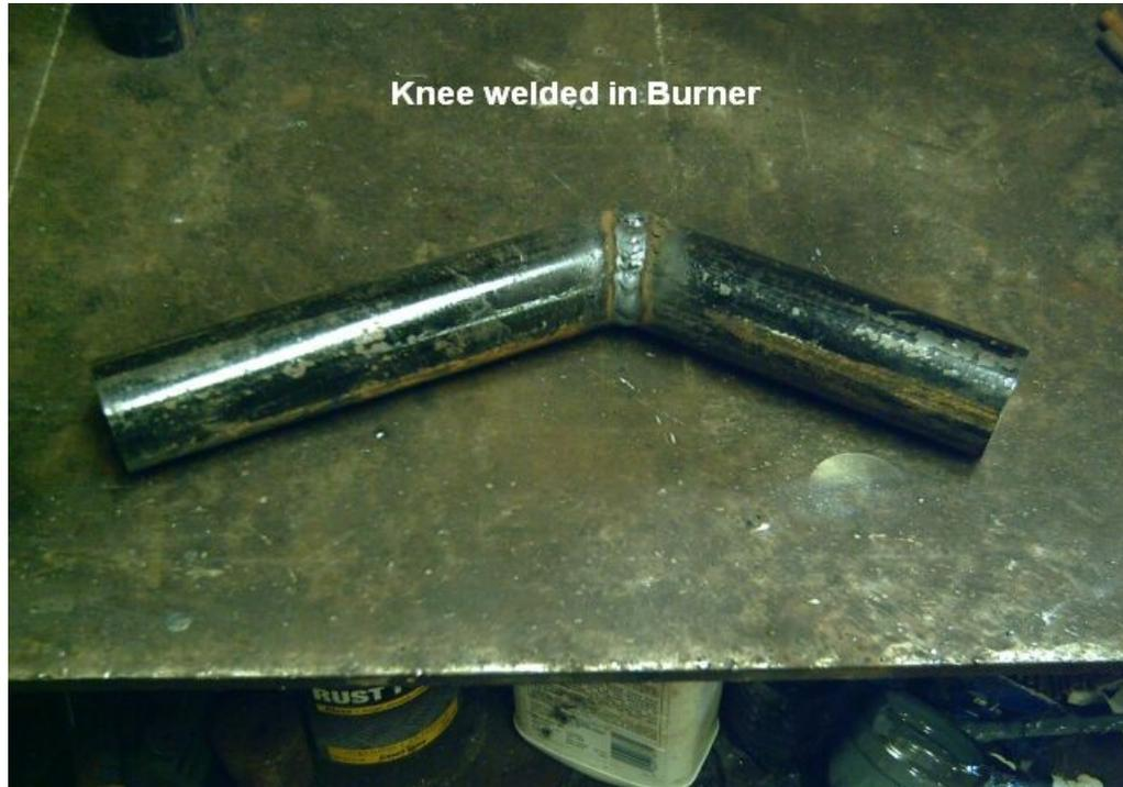
This knee construction creates a high degree of turbulence thoroughly mixing the propane and the air. This gives a more complete combustion and has an added advantage reducing the critical nature of the alignment of the orifice.
