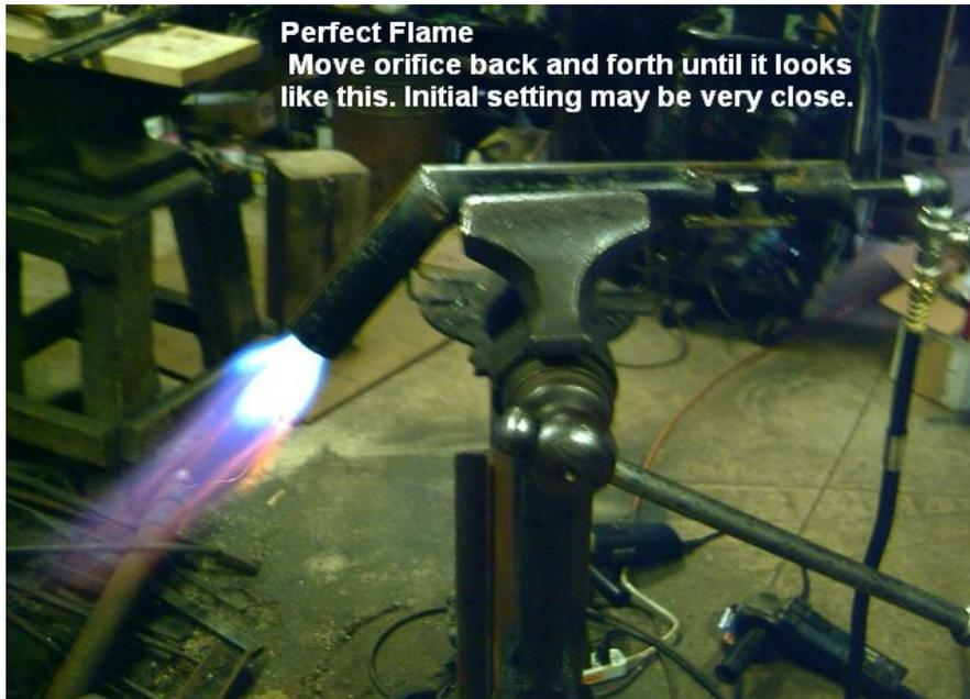
Once you get this shape and intensity of flame clamp your set screws down tight, but don't strip the threads. When tuning the burner you are looking for maximum blue flame with a minimum of yellow.
