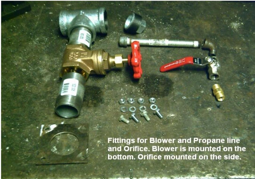
Fittings for Blower and Propane line and Orifice. Blower is mounted on the bottom. Orifice mounted on the side.
