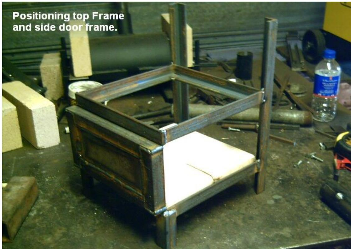
The top frame and the door are next welded together. Top frame is four 9.5 pieces of angle iron with 45 degree cuts both ends welded together to form a square. No sheet steel in this.
