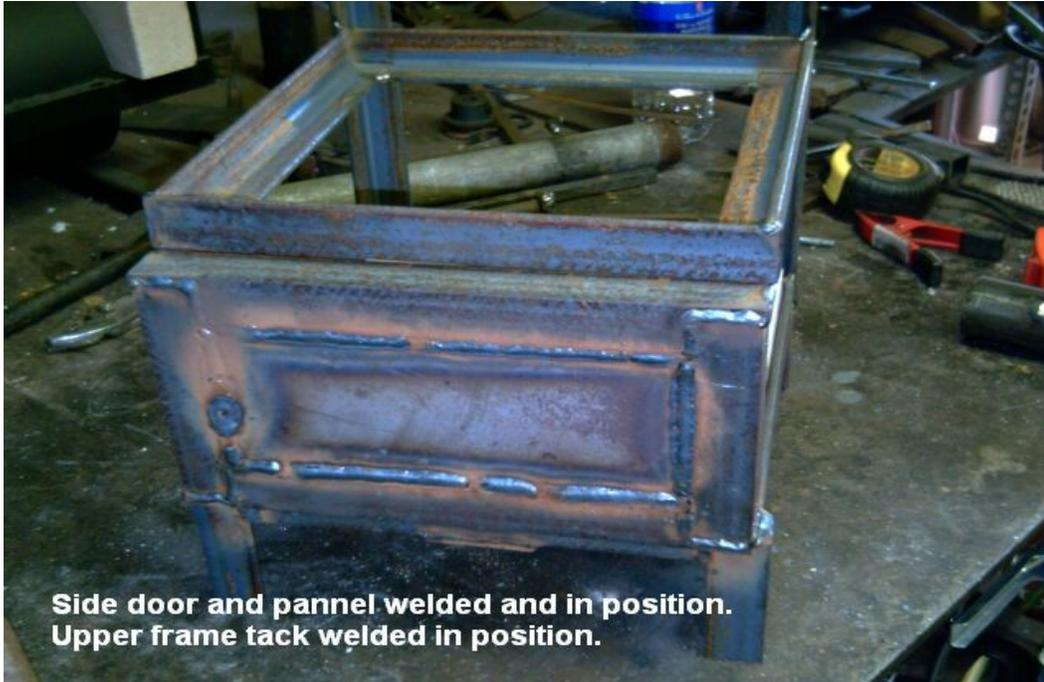
Clamp the upper frame to the tall vertical supports so that it rests  $\frac{1}{4}$  inch above the door resting on the fire brick. Use  $\frac{1}{4}$  x 1 flat bar as a spacer. Make sure the top frame is level and tack weld into position.
