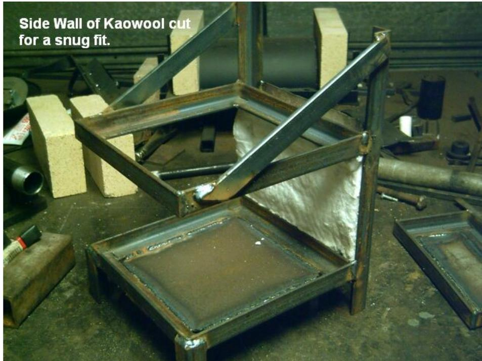
Now cut the Kaowool slightly larger than the top frame and fit in keeping it flat.
