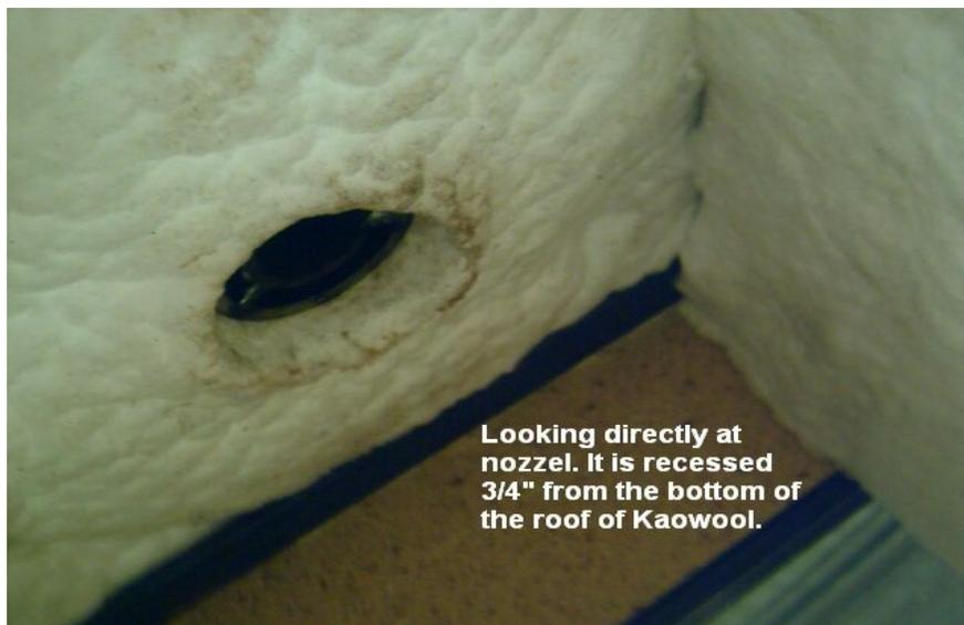
Looking directly at nozzle. It is recessed  $\frac{3}{4}$ " from the bottom of the roof of Kaowool.
