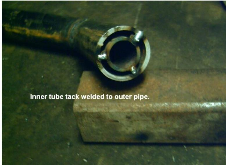
The inside short 2 inch piece of pipe really doesn't need more than just the tack welds to hold it in place since it doesn't get terribly hot. If you want to be extra confident you can drill 3 holes 120 degrees apart on the large pipe. These should match the distance of the tack welds from the end of the pipe. Then weld plug welds to secure the pipe higher up the burner. Grind all these welds smooth.
