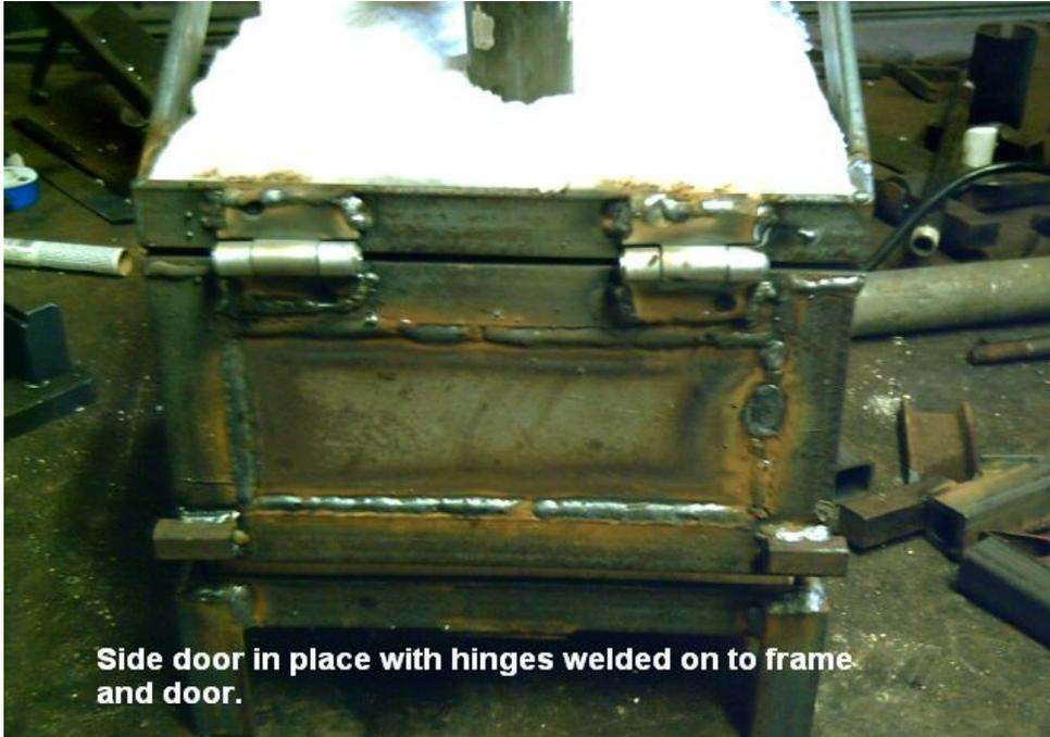
Side door in place with hinges welded on to frame and door.
