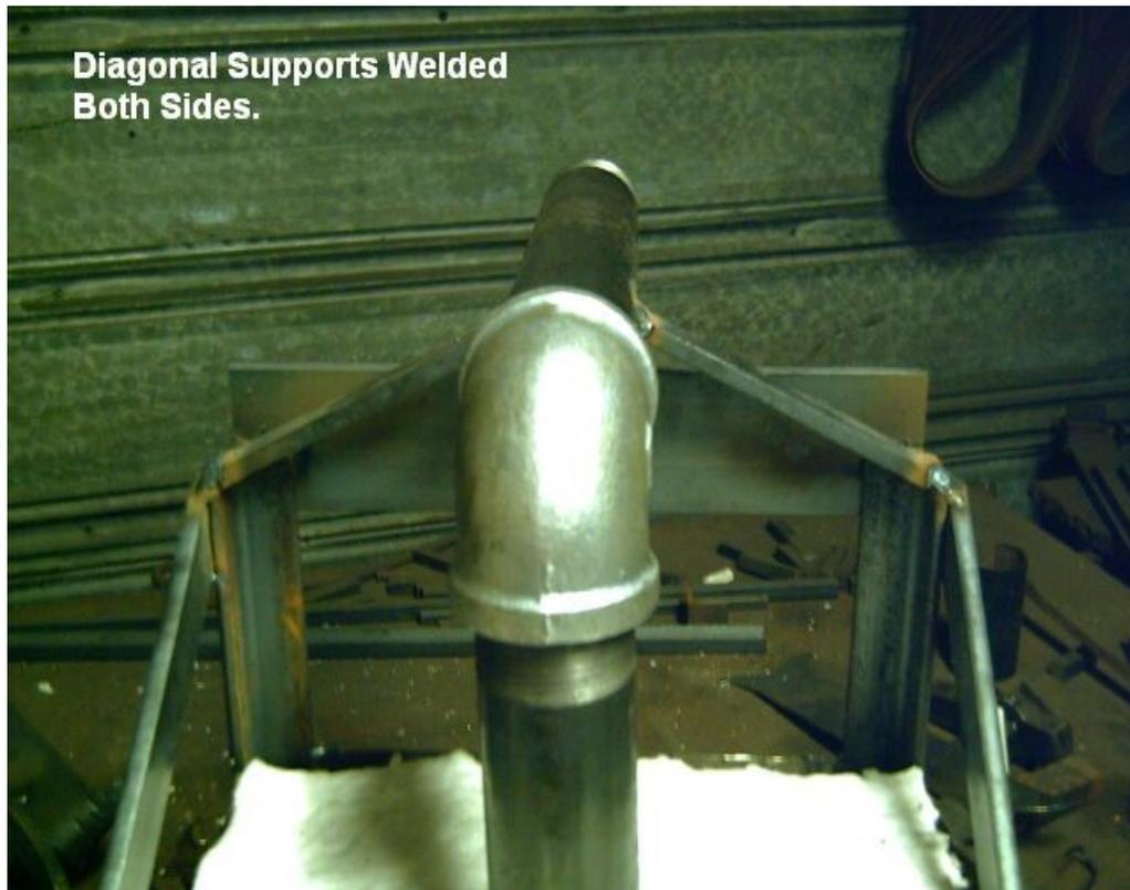
Diagonal supports on both sides of the burner tube for strength. If you ever need to do maintenance on the nozzle it simply just unscrews from the elbow.
