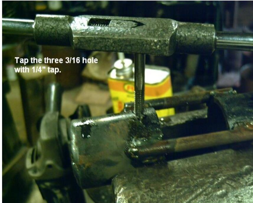
Tap the holes slowly with  $\frac{1}{4}$  inch tap. Remember  $\frac{1}{2}$  a turn reverse  $\frac{1}{4}$  turn to break off the cuttings, continue the next half turn. Make sure the tap is straight, use cutting oil. The other alternative is to drill  $\frac{1}{4}$  holes and weld nuts (with bolts threaded in them for alignment) to the out side of the pipe. I find the tapping looks cleaner. This is thin metal and taps quite easily.
