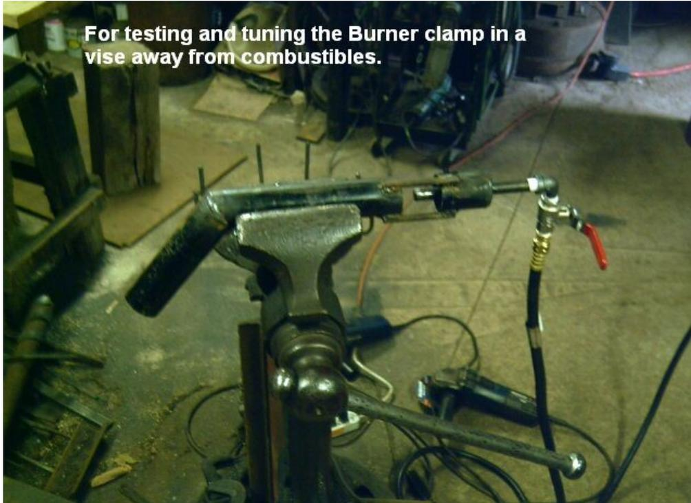
For testing and tuning the Burner clamp in a vise away from combustibles.
