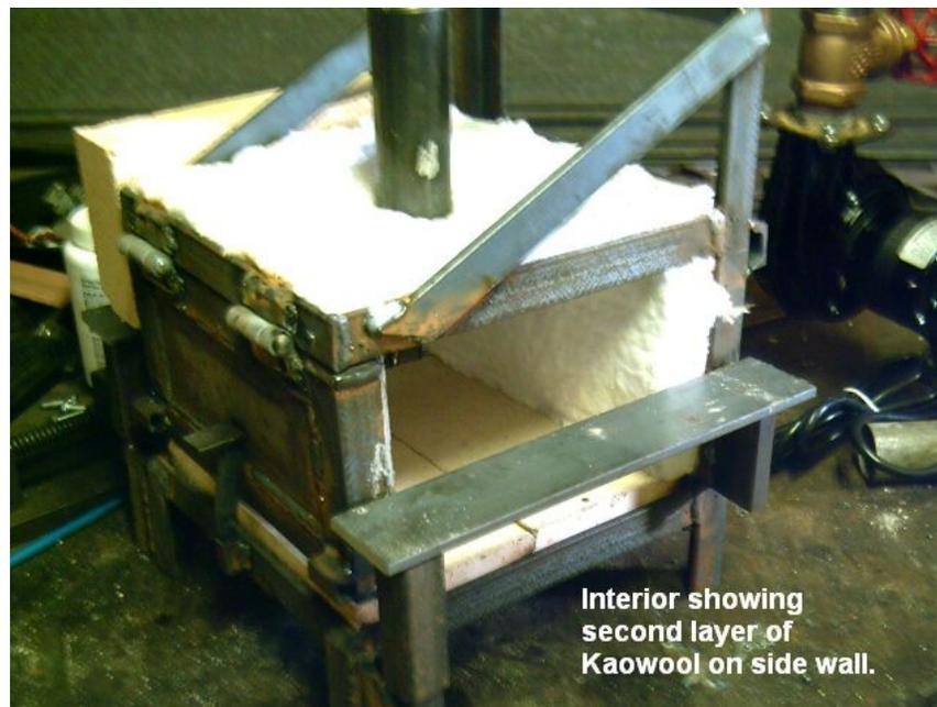
The distance between the floor of the forge to the bottom of the fire brick is 2 inches.
