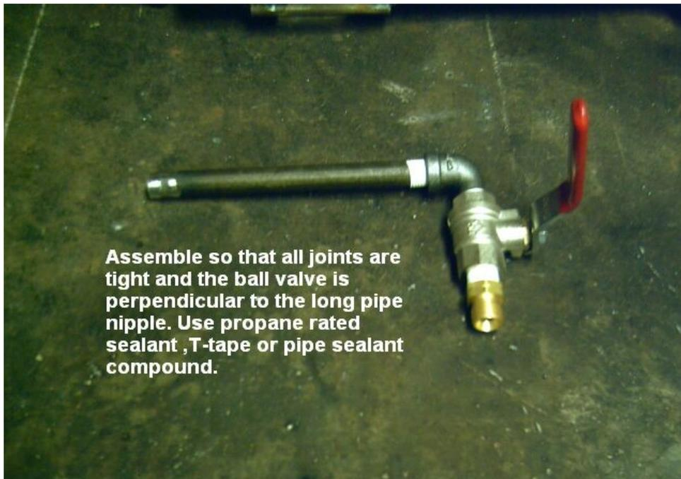
Assemble so that all joints are tight and the ball valve is perpendicular to the long pipe nipple. Use propane rated sealant, T-tape or pipe sealant compound.
