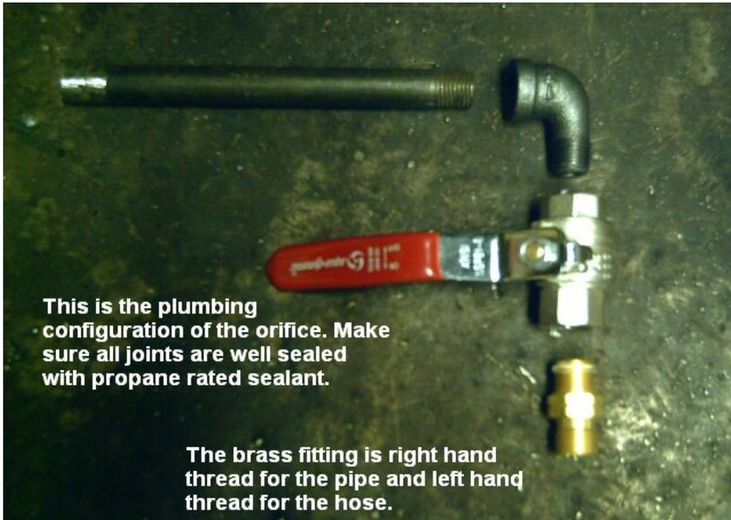
These are the components to make the orifice.
