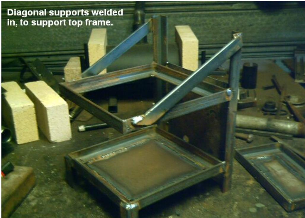
Once diagonals are in weld remaining sheet steel on to back of uprights.
