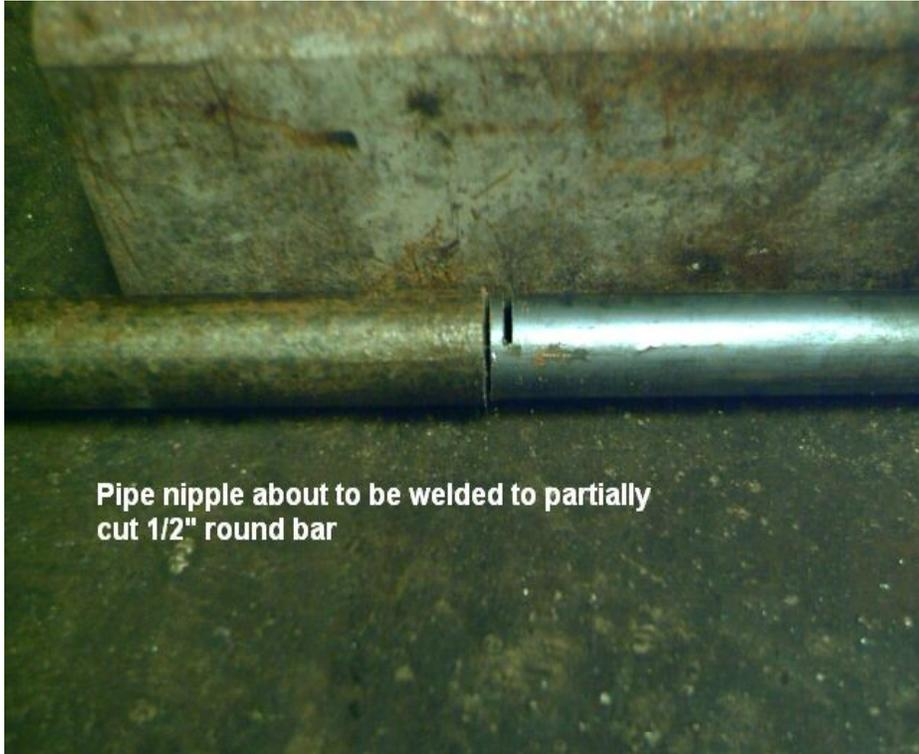
Pipe nipple about to be welded to partially
