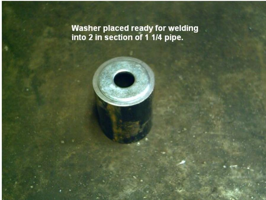
Next we set the  $\frac{1}{2}$  inch washer in the end of the 2 inch section of  $1\frac{1}{4}$  inch pipe for welding. This becomes part of the alignment for the orifice. Weld the washer into the end of the pipe keeping it square.
